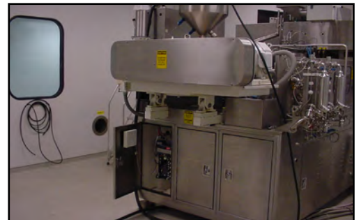
Example 1: (Blow Fill Seal Machine)
