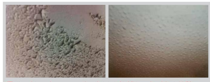
"The two pictures show epoxy coatings that started to blister and peel due to VHP."
